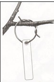
Label is tied to the branch with a 300mm length copper wire encased in a black UV-resistant PVC coating. The wire is simply twisted around itself, to form a large loop on the branch. Label size: 25mm wide X 114mm long.
